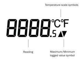
Three different functions are available on the display – most recent logged temperature, maximum logged temperature and minimum logged temperature. The push button is used to cycle through the functions. In addition, logging and alarm status are shown using two high intensity LEDs.
