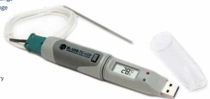
This standalone data logger measures and stores up to 32,510 temperature readings from either a K, J or T type thermocouple. A thermocouple is attached via the thermocouple socket at the base of the unit. The user can easily set up the logging rate and start-time, and download the stored data by plugging the data logger into a PC's USB port and running the purpose designed software under Windows 2000, XP and Vista (32-bit). Data can then be graphed, printed and exported to other applications.
